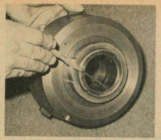
The clutch drum inner bushing support is one spot that requires beefing to eliminate all of the wobbling possible. Advanced Racing installs wider bushings on each side.
