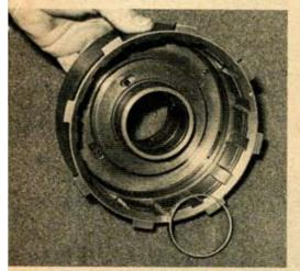
The direct clutch drum is fitted with a wider bushing of superior material, which not only prevents the drum from wobbling, but gives the sealing rings and lands much longer life. If the rings seize, a loss of line pressure will occur and the tranny may go away.
