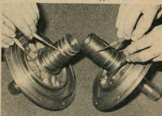
Ring land area of stator support is machined to take two improved bushings that give 65 percent better support and prevent most of the wobble inherent in single factory bushing of much smaller total surface area. Extra oiling orifices are also added to aid lubrication to the intermediate overrun band
