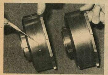
Clutch drums also receive extra oiling holes to aid in lubrication and cooling. Apply pressure is also increased for firmer shifting by modifying the oil circuits and seal system.
