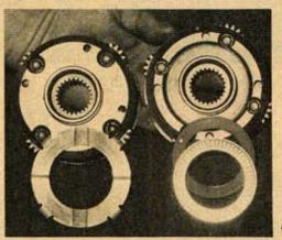
The front planetary assembly receives a new roller bearing thrust washer that reduces friction by about 65 percent over the factory babbitt thrust washer. This also reduces the heat build-up that cuts down on transmission life.
