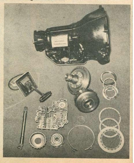
Jim Galatioto of Advanced Racing Transmissions prepares one of his "Bulldog" Turbo 350 automatics which will be set up for high-performance operation. They specialize in the 350, once considered a very marginal transmission for heavy-duty usage.
