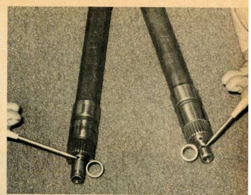
The input and output shafts receive oil lite bushings that are superior to ether babbitt or Teflon bushings. By reducing clearances they offer better support and oil pressure.
