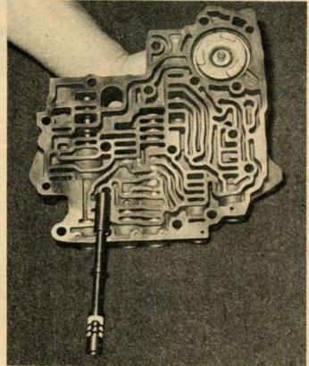
Modified valve body eliminates many troublesome parts and gives firm shifts with manual control. Shift points are fully controlled by driver, shifts are very firm.
