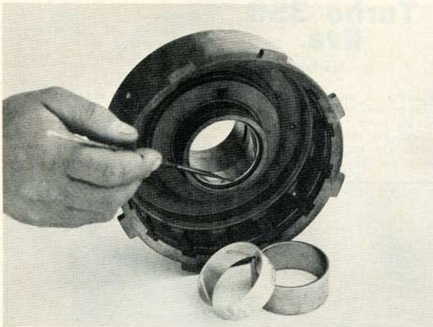
Bearing area is enlarged inside drum and new bearing is added. Top quality bushing materials are used throughout.
