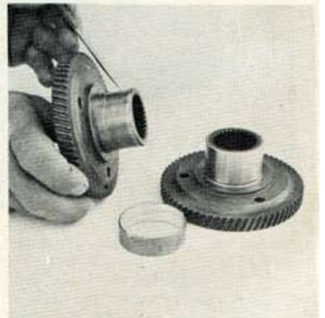
Output shaft retainer has a bushing surface which is subject to considerable wear. New retainer (right) has hard-chromed surface which eliminated problem.
