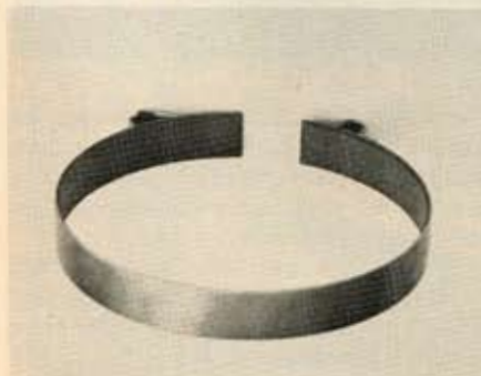
The second gear sprag is made of a brittle material which disintegrates under hard use. Replacement is a heat-treated item. Oil slots in retainer ring (pointer) are enlarged and oil flow is re-directed.
