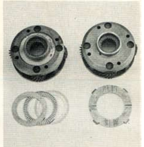
The stock babbitt thrust washer on the front planetary assembly is just one of five which are replaced with roller bearings in the Bulldog transmission, eliminating heat and wear problems.
