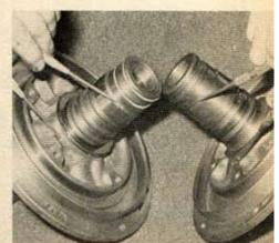
About 65 percent better support to the stator hub is achieved by special machining of the ring land area for two improved bushings. New oil holes are also added.
