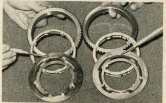
The sprag in second gear is slotted to increase and control direction of oil flow. In addition, the outer race is replaced along with the roller clutch element with heavier-duty units.
