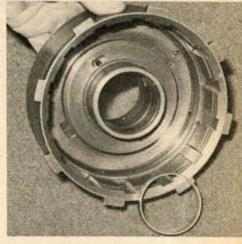
The wider bushing added to the direct clutch drum by Advanced gives the sealing rings and lands increased longevity and also prevents the drum from acquiring a wobble from wear. Some 350s have been known to suffer ring seizure, causing line pressure to drop and the ultimate loss of the transmission.
