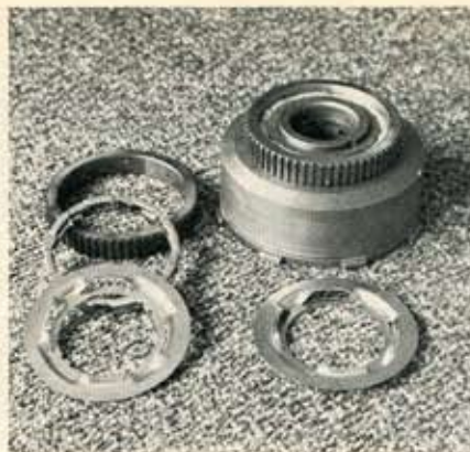
LEFT—Jim uses heat-treated sprag race (stock one cracks), and latest Bulldogs will have a new Borg-Warner 36 element sprag—strongest one now available. Retainer ring (bottom) is also slotted to provide extra oiling.
