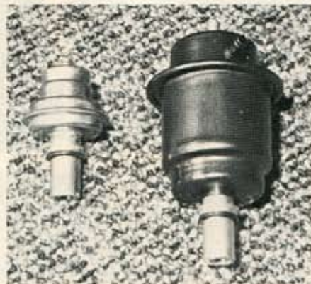
ABOVE—Of course all of the clutch discs and the band are replaced with improved components made with tougher wearing surfaces. LEFT—In case you've got cramped quarters around the tranny, this new mini vacuum modulator (left) helps out.
