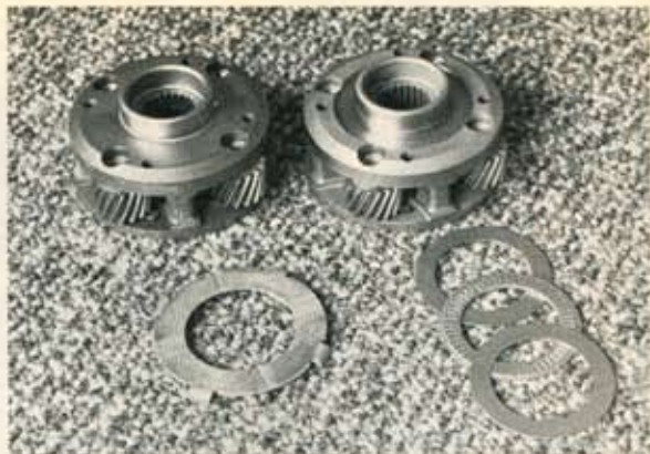
RIGHT—A large groove is cut in the front planetary to allow substitution of roller bearing (right) for the stock babbit thrust washer.
