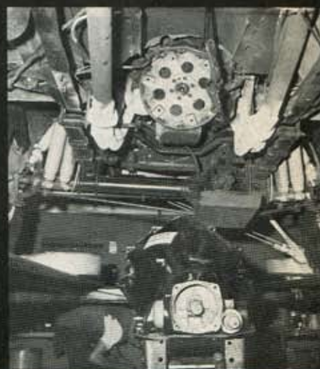
24. The Advanced Transmissions Bulldog tranny is ready to be lifted into place. The stock flywheel is used and standard mounts hold the strongbox in place.
