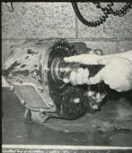
16. With the drive gear up fully against the sleeve and the teeth aligned, turn the drive gear. It should turn freely without binding.
