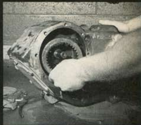
12. With the new gear and bearing in place, the gear sleeve is slipped in against the gear, with the shifting forks in place on the sleeve.
