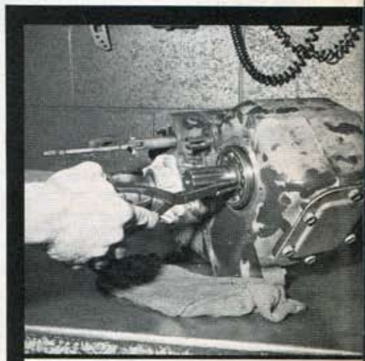
7. The snap ring retaining the bearing on the input shaft must be removed. Using the proper tool will prevent damage and temper tantrums.
