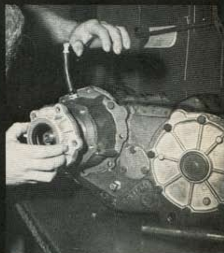
18. When the bearing housing is installed and you're sure that no bearings have fallen out, replace the bearing retainer and tighten down the bolts.
