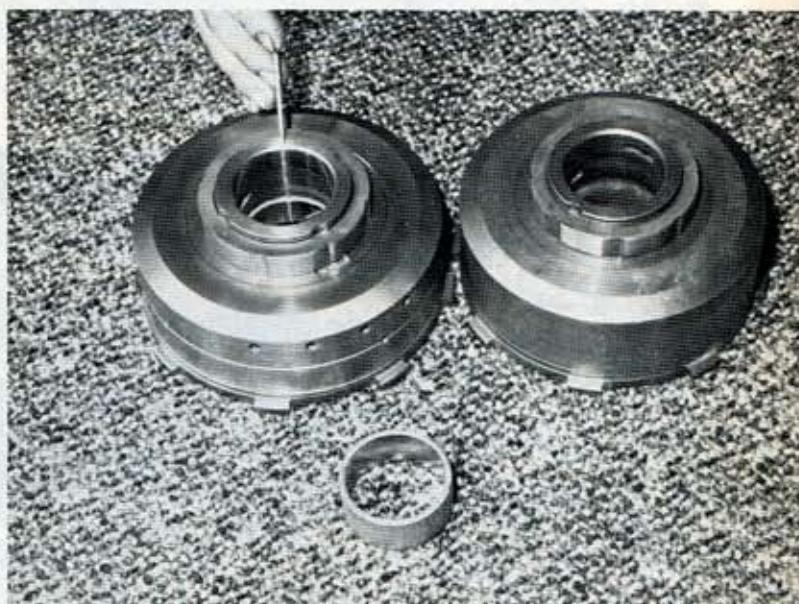
ABOVE—The Bulldog bushings are also made of a tougher grade of metal than the originals. Jim states that the latest stock Turbos are now even using Teflon instead of metal for bushings.
