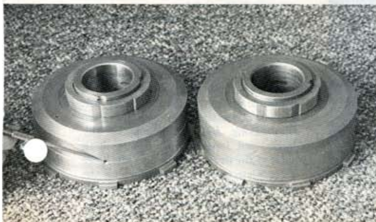
Jim also believes in providing as much increase in oil flow as possible for lubrication as well as cooling. He turns a groove in the clutch drum and drills four small holes in its circumference to help cool the one band in the trans.
