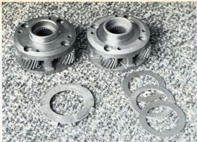
ABOVE—It takes about one second to see how much more efficient a roller bearing is than a babbitt thrust washer. Large groove must be turned in front planetary housing to allow substitution. RIGHT—The components which take the most direct abuse in any automatic are the clutches and bands. The Bulldog, of course, uses the toughest materials available.
