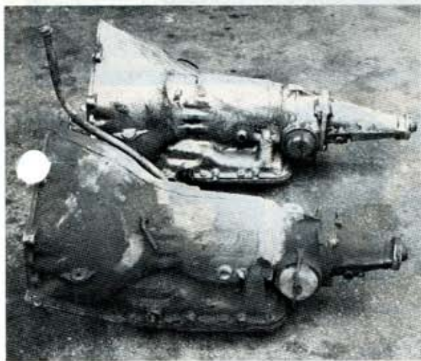
ABOVE—Big advantage of T-350 is that it's the same size as the 2-speed Powerglide. However, units with longer tailshafts are available. Cores, like these, aren't expensive. RIGHT—Jim recommends a rod-linkage shifter, like the Mustang. BELOW—And when it comes to truckin' with a Bulldog 350, Jim knows how well they work — his four-by-Chevy has one.
