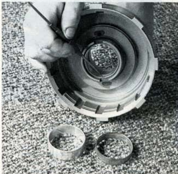
Jim also believes in providing as much increase in oil flow as possible for lubrication as well as cooling. He turns a groove in the clutch drum and drills four small holes in its circumference to help cool the one band in the trans.
