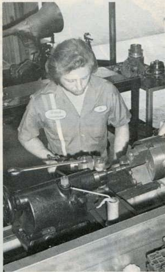
LEFT—Another weak spot in the 350 is the support for the input shaft, upon which rides the pump shaft and clutch drum assembly. Besides adding beefier bushings, Jim also machines the shaft (below) for extra oiling. Plenty of lathe time goes into a Bulldog!
