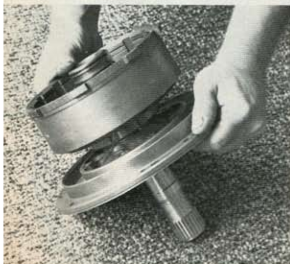
Jim found the main problem with the 350 to be poor support of the high gear/reverse clutch drum on the front pump shaft (left) causing it to wobble. Solution (above) is a complete new wide-bearing sleeve pressed over turned-down shaft.
