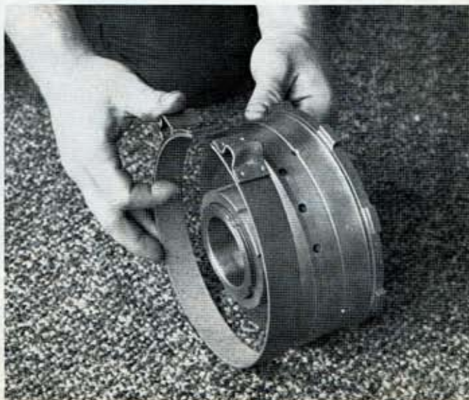
ABOVE—The Bulldog bushings are also made of a tougher grade of metal than the originals. Jim states that the latest stock Turbos are now even using Teflon instead of metal for bushings.
