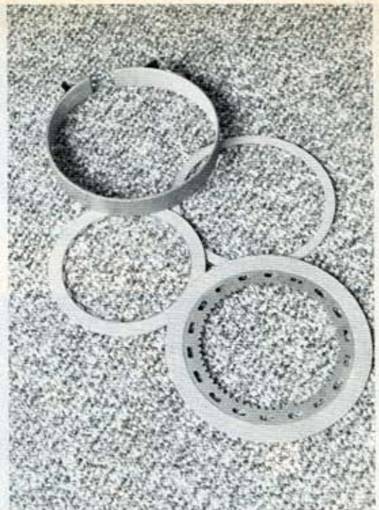
ABOVE—It takes about one second to see how much more efficient a roller bearing is than a babbitt thrust washer. Large groove must be turned in front planetary housing to allow substitution. RIGHT—The components which take the most direct abuse in any automatic are the clutches and bands. The Bulldog, of course, uses the toughest materials available.
