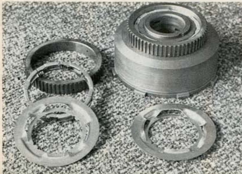
BELOW—In stock 350's the sprag race has been known to crack. Jim uses a special heat-treated sprag (shown at center, left), and latest units will use new B-W 36-element sprag. Retainer ring is slotted for extra oiling.
