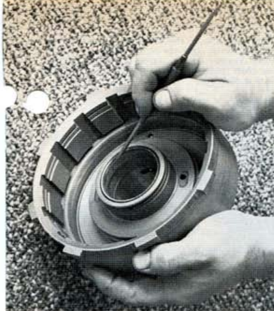
ABOVE—This is how Jim found most stock bearings in used 350 drums—chewed up. BELOW—He machines wider lands in the drum to accept his own special bushings, front and rear. Contrast between two is evident in photo below.
