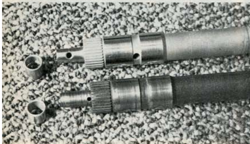
BELOW—In stock 350's the sprag race has been known to crack. Jim uses a special heat-treated sprag (shown at center, left), and latest units will use new B-W 36-element sprag. Retainer ring is slotted for extra oiling.
