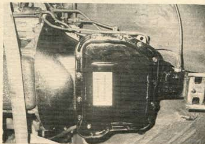
Installed, the Advanced transmission eliminated all the slippage and leakage problems we had experienced in our Dodge. An auxiliary cooler is the next recommended step for maximum transmission longevity.
