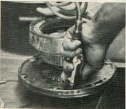
Pressure is used to test clutch position in the direct clutch.
