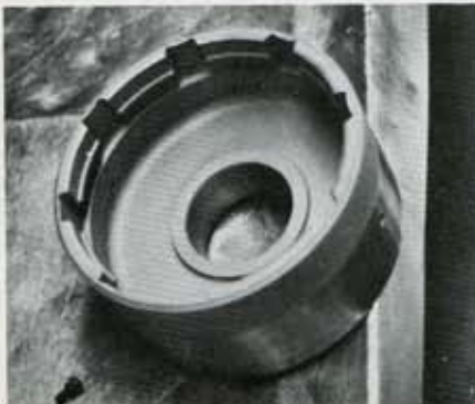
The reverse drum is drilled to add more oil from the main shaft to the rear band.
