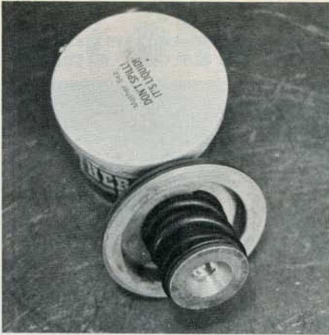
Reverse band-apply piston before removing spring.
