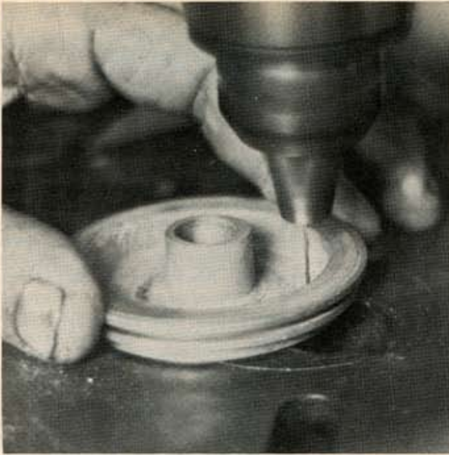
Reverse piston is drilled to release 25 percent of the pressure to prevent band breakage.
