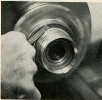
The support ring is hand shaped with a file.
