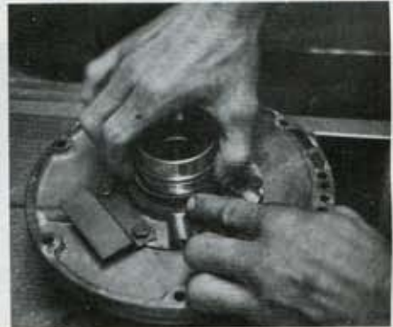
Installing the sealing rings for the direct clutch drum.
