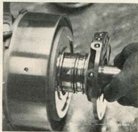
The reaction shaft support ring must fit the I.D. in the direct clutch drum within specs.
