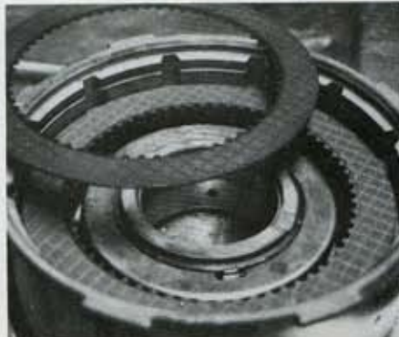
Raybestos clutch material is used in the direct clutch.
