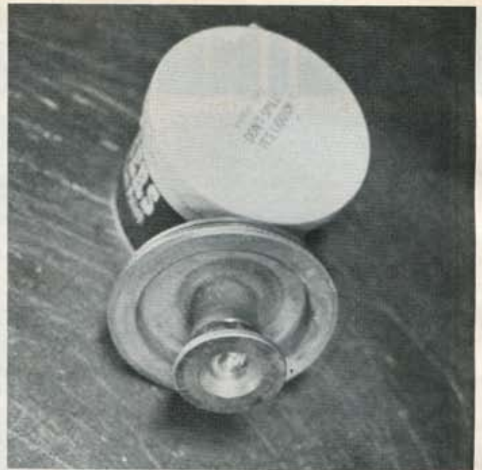
Reverse piston spring is removed to stop lock-up from manual low to 2nd gear.
