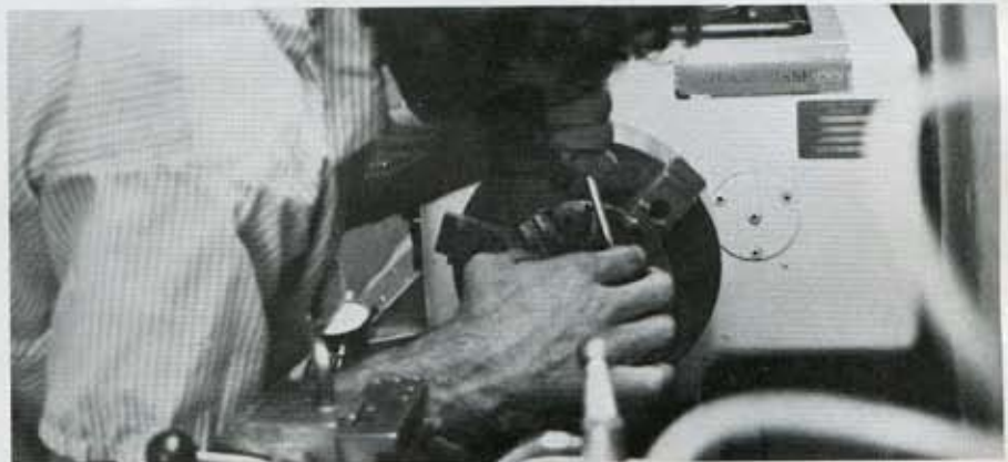
Reaction shaft is machined to accept the Teflon ring.
