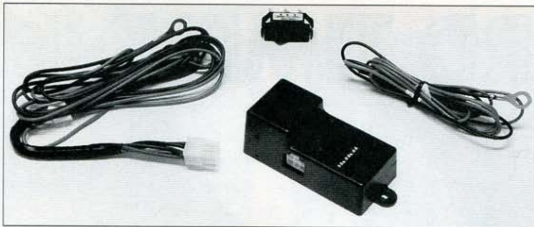
This Rostra Lockup Delay Module can be easily installed on Ford trucks to have the E4OD converter clutch lockup triggered by vehicle speed instead of throttle position. It can be set in 5-mph increments, from 30 to 50 mph.
