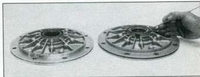
ATO's improvements to the E4OD start right at the beginning of the front pump. A groove is machined into the cover to enable a locking seal retainer (right) to replace the crush-fit factory front seal, eliminating a potentially major hazard.
