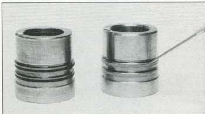
Special-formulation Teflon rings replace the stock, cast-iron sealing rings on the center support housing. Virtually frictionless, the Teflon rings provide positive sealing, better heat resistance, and long life. When the OEM rings wear out, the pressure used to apply the 3rd gear piston drops, resulting in slipping and burned clutches.
