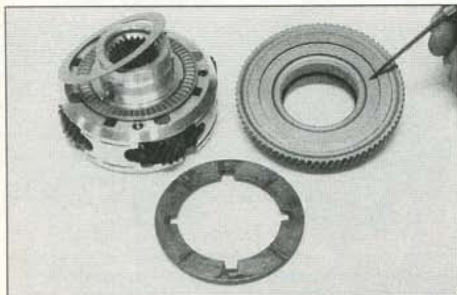
Shown here is the machining performed on the front planetary to create the clearance and register to hold the new thrust bearing in place. In the foreground is the stock thrust washer that is replaced.
